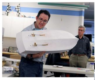
**Bryan Morse** brought in his Dumas Dauntless model which is now sealed with shafts, struts and props attached. He plans to power it with twin speed 850s. Since he lives in an apartment he is contemplating a vertical stand to take up less room. **Dr Ron** showed the mold lifted from the plug he brought in last month which is now ready to lay up a hull having 7 coats of parting wax and an application of PVA.
