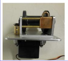
The winch is fully operational and powered by a standard servo that can be connected directly to a proportional channel.
