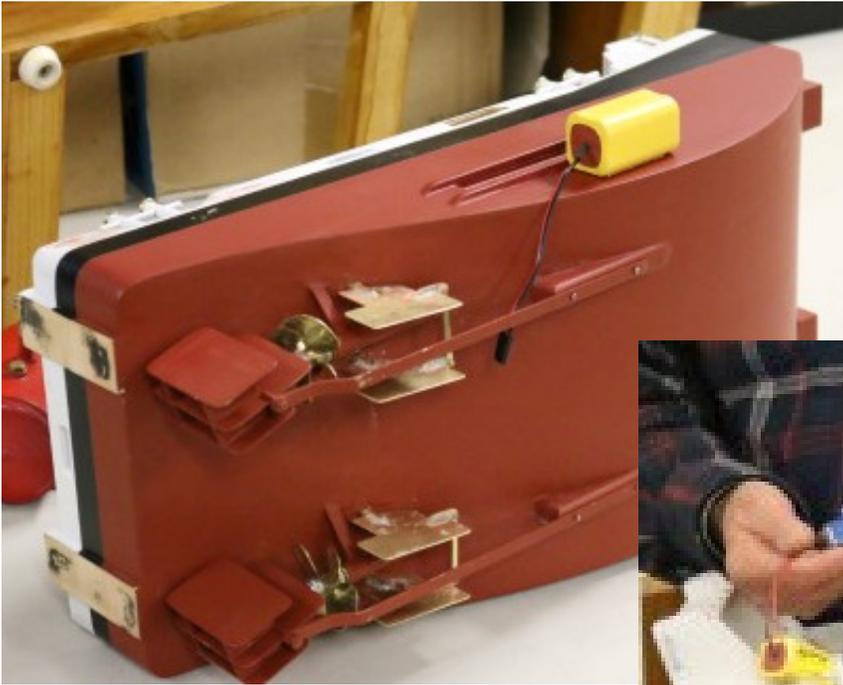
**Bob Wickham** demonstrated how he constructed the forward rudders to act in unison with the rear rudders, the posts of which penetrate the hull to be connected to the rudder horn and servo. There was not enough room in the hull to put in forward penetrating rudder posts. The dual prop super springer is really looking cool.
