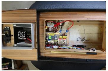
sound and a very good sounding small German speaker under the hatch cover but it makes the boat quite full so I am still thinking about that. Because the gear drive is quite noisy already, it also needs a voltage buck boost transformer since it will only run on 12 volts and the boat is set up with 6 volts.
