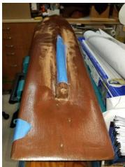
It appeared there was not enough clearance in the stern for the rudder steering arm, so I used a router bit and rasping bit to make room. I used a 2 in hand rasping sander to remove as much of the black material before I had to stop working due to injuries from a serious bike crash a month ago.
