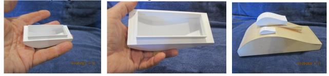
Paul talked about the problem encountered when reducing a larger CAD 3D model down to a size to fit on his 3D printer. As the model is reduced, the wall thickness got so thin that he could not print the model. The model was "Victualling Inshore Craft VIC RC Cargo Ship, scale 1/35, and designed by Askarsi. This nice model was 730 mm (29 inches) long and Paul wanted to reduce the length to 180 mm (7 inches). This is a common problem with using another person's model and changing the 3D print size.
