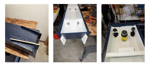
I made the egg crate boards from leftover wainscoting boards to keep the water ballast from sloshing around.
