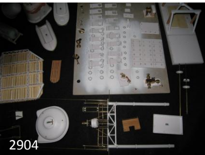
All the small parts were assembled as per the plans and secured to a piece of cardboard with a glue stick ready for painting. See pictures 2903, 2904, 2906, 2907, 2908, 2809, 2910, 2928, and 2829.
