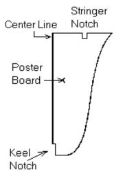
Transferring template patterns to plywood bulkheads is accomplished by placing pattern on your plywood tracing the outline with a pencil
