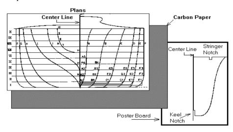
Using a sharp Xacto knife or scissors cut out each pattern. For straight edges using a metal ruler aids in cleaner cuts.
