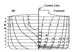
Also mark your keel and stringer notches. Typical keel are plywood with widths
