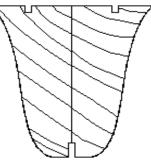
Once all the bulkheads are cut out, you can start the frame assembly. The assembly starts with a building board on which the keel and bulkheads are attached. It is imperative that this "base" be very true (No bends or warps) and if needed be braced to prevent warping once the assembly has started. This base should be constructed from 3/4" plywood and if the model is long (>??") in size then additional bracing may be needed as shown.
