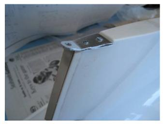
A piece of aluminum replaced the plastic one intended to fix the rudder to the bottom of the hull piece. The tail end of the hull, which was a separate ABS piece, was glued with Weldon Scigrip 16 acrylic cement. The joint edges were faired with epoxy putty.
