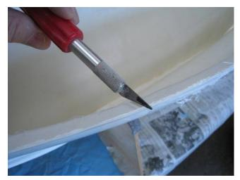
The excess ABS on the hull, deck and bulwarks was cut near the line with heavy shears and the scraped with a knife blade and sanded.
