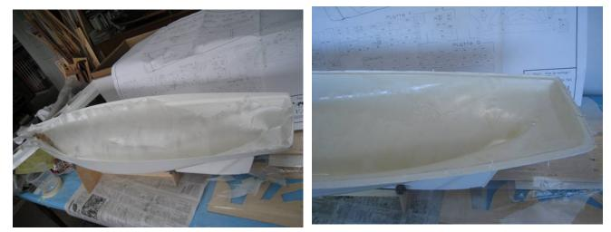
After building the stand to support the hull, I decided to reinforce the hull with fiberglass cloth and epoxy resin for added strength.
