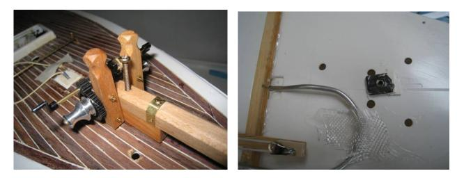
Brass rings provided for the bowsprit and mast construction were the wrong size, so they were made from brass tubing of the appropriate sizes using a cut off saw.
